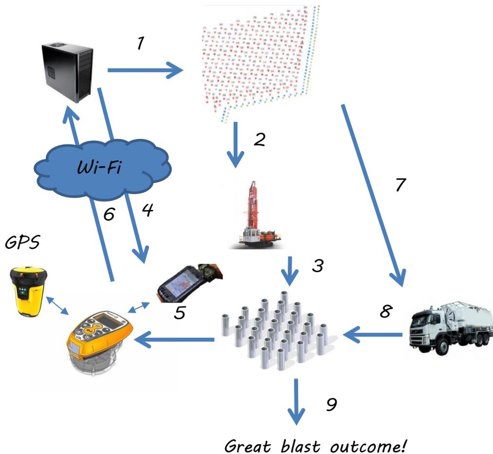
Figure 5 : Example 4, System deployed with Visualisation Module and High Precision GPS.
